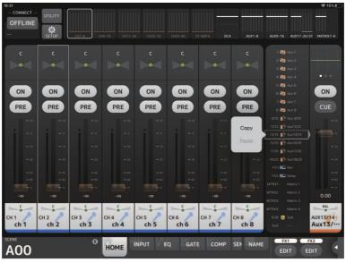
In SENDS ON FADER mode, the details area changes to display SENDS ON FADER information. Note, however, that the display does not change for channels that have no send destination.
