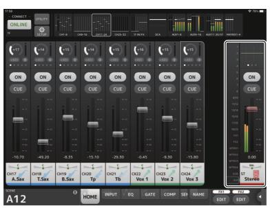
The STEREO channel strip is normally displayed in the overview strip area. When using SENDS ON FADER mode, the destination AUX channel, SUB channel, or MATRIX channel strip is displayed here.
