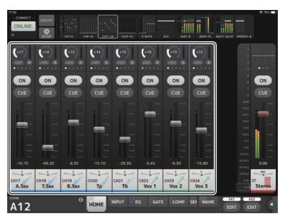
Channel strips for 8 channels are displayed in the details area. You can scroll left and right to display the channel strips for other channels by swiping left or right on an inactive area of the screen.
