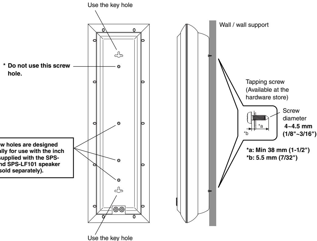
Fasten screws into a firm wall or wall support as shown in the figure, and hang the holes of the rear of the speaker on the protruding screws.
