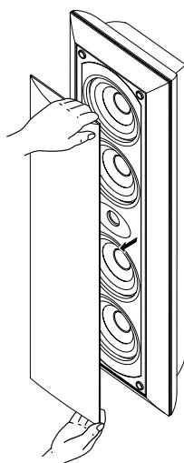
The front cover is fastened to the enclosure at four points and can be removed if desired. To remove the cover, hold on to both sides and slowly pull straight away from the speaker. To reattach, line up the four holes on the inner surface of the cover with the four corresponding pegs on the speaker and push gently.
