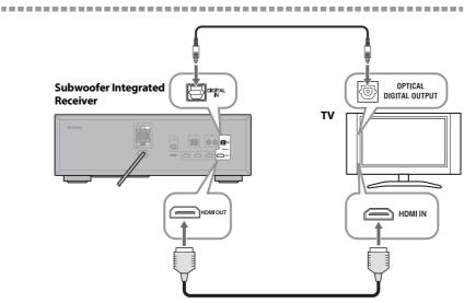
Connect your TV's HDMI jack to the HDMI OUT jack of the Subwoofer Integrated Receiver, using an additional HDMI cable, as shown.
