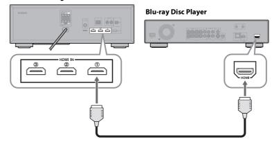
If your TV is HDMI-capable, you can connect it and Blu-ray Disc Player via the Subwoofer Integrated Receiver. Using the supplied HDMI cables, connect the Blu-ray Disc Player's HDMI output jack to the HDMI IN (1) jack on the Subwoofer Integrated Receiver, as shown.
