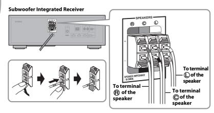
Connect the speaker cable to the Subwoofer Integrated Receiver. Be sure to insert the cable by matching the wire color with the color-coded terminal on the rear panel.
