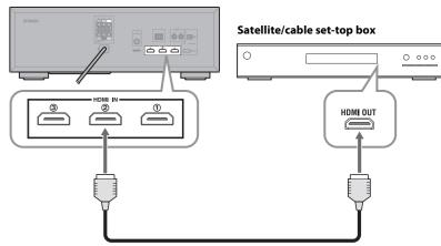
Use an additional HDMI cable to connect your satellite/cable set-top box to the Subwoofer Integrated Receiver's HDMI IN (2) jack, as shown.
