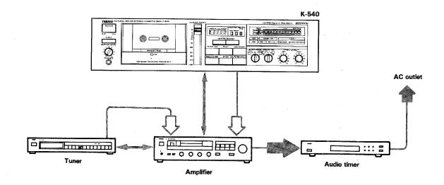
When using the AUTO MODE selector in combination with a commercially available audio timer, it is possible to make recordings and initiate playback at any time automatically by presetting the deck in advance.
