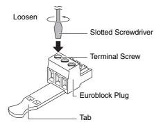
\* The following explanation uses a Euroblock plug that features a tab as an example.
