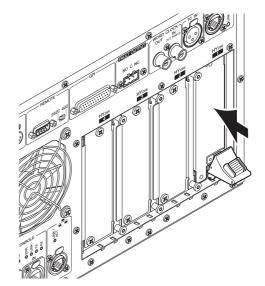
**4.** Pull up the card installation lever to lock in the card.
