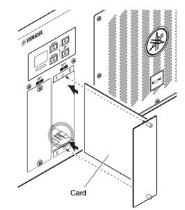
**4.** Fasten the card using the screws attached to the card.
