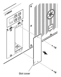
**3.** Align both edges of the card with the guide rails inside the slot, and then insert the card into the slot.
