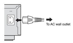
Plug the power cable into the AC IN, then plug the power cable to an AC wall outlet.
