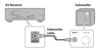
Use the included subwoofer cable to connect the subwoofer's INPUT jack to the AV Receiver's SUBWOOFER jack. See "Using the subwoofer" on page 6 for more information about the subwoofer and its operation.
