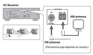
Connect the AM loop antenna and indoor FM antenna to the AV Receiver, as shown. See the AV Receiver's owner's manual for more information about connecting antennas.
