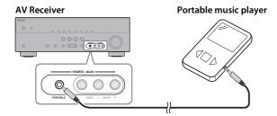
Use a 3.5 mm stereo mini plug cable (not included) to connect your portable music player to the AV Receiver's PORTABLE jack (on the front panel), as shown.
