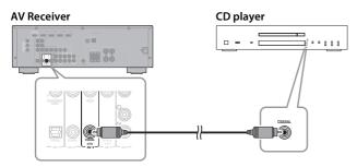
Use an audio pin cable (not included) to connect your CD player to the AV Receiver's AV 3 COAXIAL(CD) jack, as shown.
