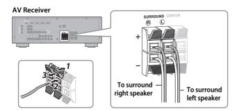
Connect the surround speaker cables to the AV Receiver. Make sure you connect the speakers with the correct polarity: positive (+) terminals to positive (+) terminals, and negative (-) terminals to negative (-) terminals.
