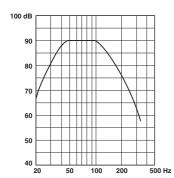
The following graph shows the combined frequency characteristics of the subwoofer (NS-SW280) and front/center speaker (NS-BR300), and surround speaker (NS-B285).
