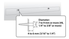
3 Hang the speaker by its keyhole slots onto the protruding screws.
