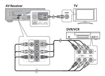
Use a video pin cable (not included) to connect the AV Receiver's MONITOR OUT jack to a composite video input on your TV, as shown.
