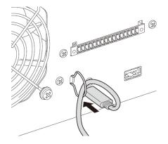
3. Pass the USB cable through the hook, and then connect it to the USB port.
