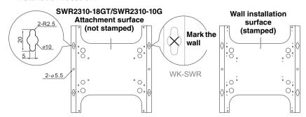
2. Provisionally attach four commercially available screws to the locations that you marked in step 1.
