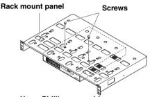
Use a Phillips screwdriver to firmly fasten the screws.
