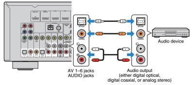
If you select the input source by pressing AV 1–6 or AUDIO, the audio played back on the audio device will be output from the unit.
