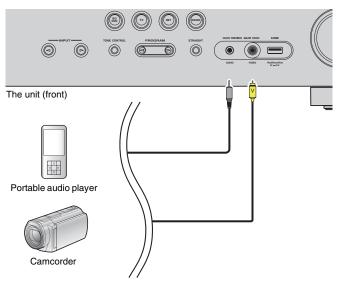
If you select "V-AUX" as the input source by pressing V-AUX, the video/audio played back on the device will be output from the unit.
