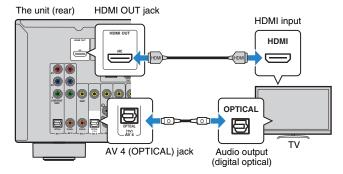
If you switch the input source of the unit to "AV 4" using the AV 4 or SCENE(TV) keys, the TV audio will be played back on the unit.
