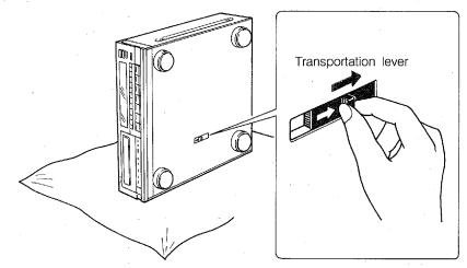
When the transportation lever is not set in the direction of the arrow, the unit does not start playing.
