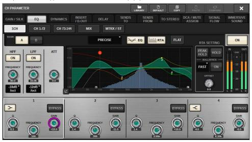
You can switch between popup windows using tabs as needed. Some popup windows show several buttons called "tool buttons" at the top of the window. You can use these tool buttons to recall libraries or to perform copy and paste operations. Press the "x" symbol located in the upper right corner to close the popup window and return to the previous screen.
