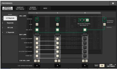
For more information on the settings, refer to the SURFACE SETTING1 screenof the Preferences Settings. The selected layer will be indicated by a bold white frame in the meter area. Also, the layer of the linked bay will be indicated by a thin white frame.
