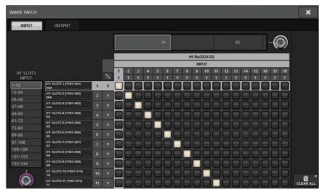
Specify the patching that will be input from the I/O rack to the Dante-enabled HY card.
