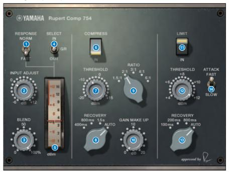
METER RESPONSE switch Selects the meter response speed.
