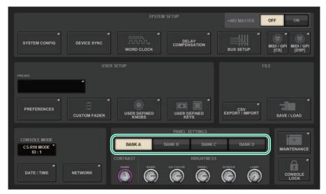
2 In the field located on the bottom row of the SETUP screen, press one of the BANK A-D buttons.
