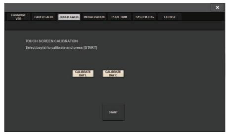
4 Press the CALIBRATE BAY L button to calibrate the left touch screen panel. Press the CALIBRATE BAY C button to calibrate the right touch screen panel.
