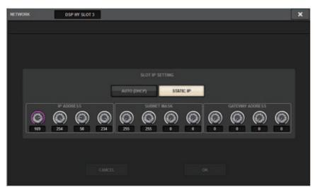
AUTO (DHCP)... The. IP address is obtained automatically.
