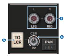
In the TO STEREO popup window, if the PAN/BALANCE select button is set to PAN, the L and R PAN knobs are shown, enabling you to specify the panning of the signal. If you use the ST/LCR mode select button to select LCR, the LCR button and CSR knob appear. The LCR button turns on/off the signal that is sent from the channel to the STEREO bus, and the CSR knob specifies the level ratio between the signal that is sent to the STEREO A (L/R) bus and to the STEREO B (C) bus.
