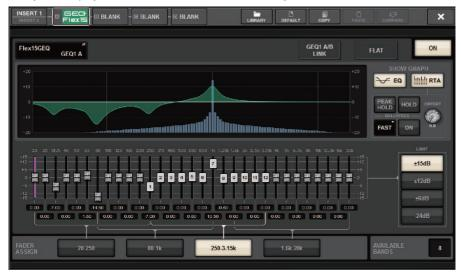
This window is the same as that for the 31BandGEQ, except that the AVAILABLE BANDS field is a real-time indication of the number of additional bands (maximum 15) that can be controlled for the current GEO.
