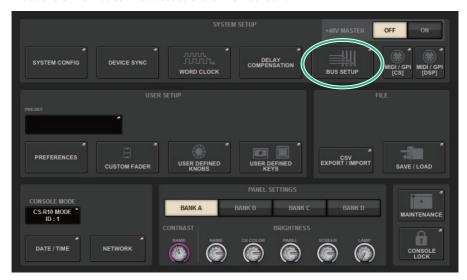
2 Press the BUS SETUP button to open the BUS SETUP popup window.
