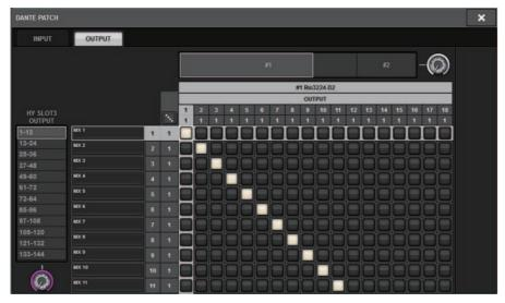
Specify the patching that will be output from the Dante-enabled HY card to the I/O rack.
