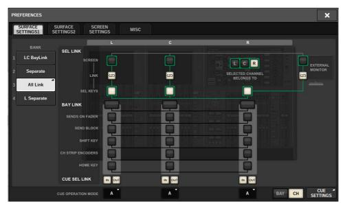
**Separate...** This option is another simple setting. You can select a different channel for each bay. Up to three channels can be viewed and controlled simultaneously.
