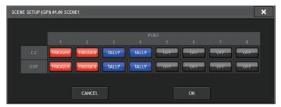
4 For each scene, specify the control signal that you want to output to each GPI OUT port.
