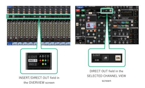
The "INSERT/D.OUT popup window (1CH)" (p.513)appears There are two types of INSERT/D.OUT popup window: 1CH and 12CH D. OUT.
