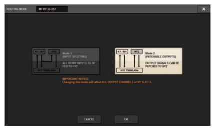
This window enables you to switch the routing mode for HY slot 2.
