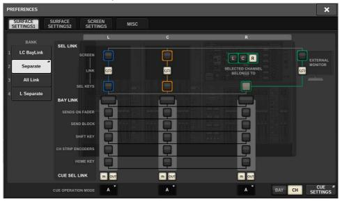
**L Separate**... This option is suitable for two operators. For example, operations on bay (L) will not interfere with the operations on bay (C&R).
