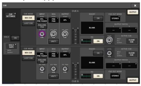
2 Use the CUE MODE buttons to select either the mode in which channels are mixed for monitoring, or the mode in which only the last-selected channel is monitored.
