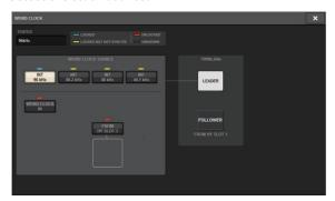
The default value is 96kHz. If the unit is operating correctly with the selected clock, the indicator for the selected clock will light blue, and the clock frequency will be displayed in the upper left of the LEADER CLOCK SELECT field.
