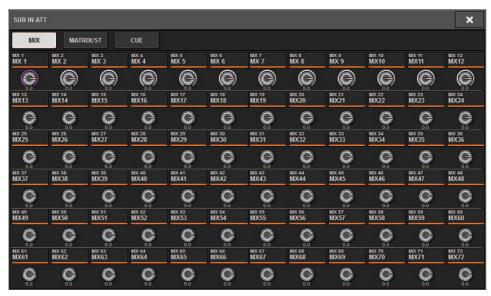
Use the tabs to select an output channel, and use the knobs to adjust the gain for each channel.
