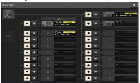
When connecting PM Editor, you must specify the data sync direction for the DSP engine.
