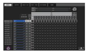
3 Use the knob in the upper right to display the desired input port.
