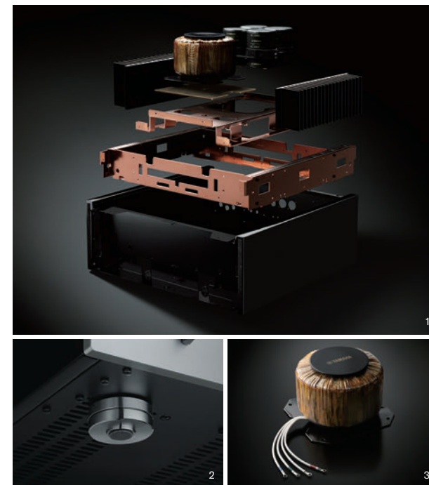
[1] Innovative chassis with rigid streamlined construction and Mechanical Grounding, which is applied to massive and heavy parts subject to vibration, such as power transformers and block-capacitors. [2] Newly developed feet of cut brass employ a screw-in structure with separate upper and lower sections that incorporate a spike at contact point, provide both pinpoint support and protection. [3] Massive toroidal power transformer with combined left/right capacity of 1200 VA maximises the overwhelming power and strength of the low-frequency sound.
