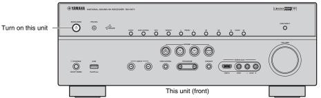
Before connecting the power cable (General model only) Make sure you set the switch position of VOLTAGE SELECTOR according to your local voltage. Voltages are AC 110-120/220-240 V. 50/60 Hz.
